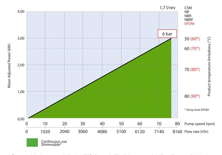
Flows are typical and were measured with water at 20 °C with no suction lift or discharge pressure. Actual flows will vary according to suction conditions, discharge pressure and normal component production tolerances.
