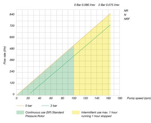
Flows are typical and were measured with water at 20°C with no suction lift or discharge pressure. Actual flows will vary according to suction conditions, discharge pressure and normal component production tolerances.
