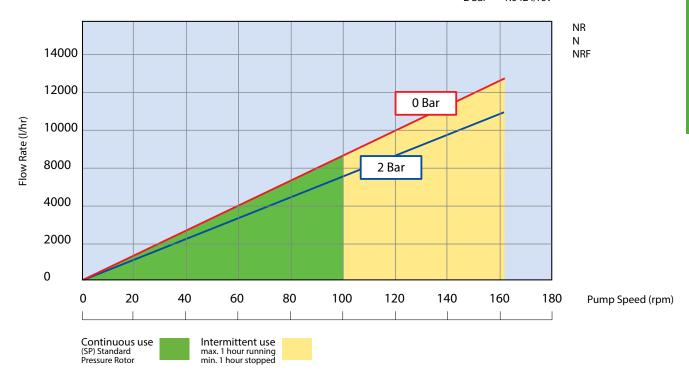
Flows are typical and were measured with water at 20°C with no suction lift or discharge pressure. Actual flows will vary according to suction conditions, discharge pressure and normal component production tolerances.
