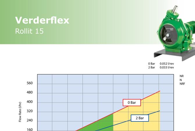
Flows are typical and were measured with water at 20°C with no suction lift or discharge pressure. Actual flows will vary according to suction conditions, discharge pressure and normal component production tolerances.
