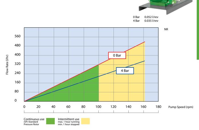
Flows are typical and were measured with water at 20°C with no suction lift or discharge pressure. Actual flows will vary according to suction conditions, discharge pressure and normal component production tolerances.
