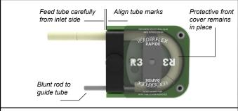
Figure 8 Tube assembly - EV 3000
