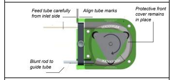
Figure 11 Tube assembly - EV 8000
