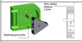
Figure 12 Replacing the rotor - EV 8000
