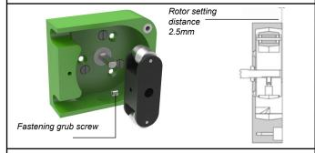
Figure 9 Replacing the rotor – EV 3000
