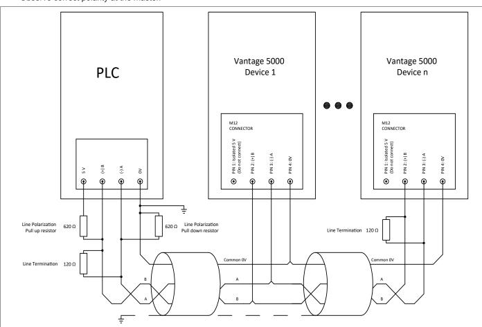
Figure 4 Modbus<sup>®</sup> system wiring diagram
