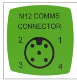
PIN 1: Isolated 5V (Do Not Connect) PIN 2: B (+) PIN 3: 0V PIN 4: A (-) PIN 5: NC
