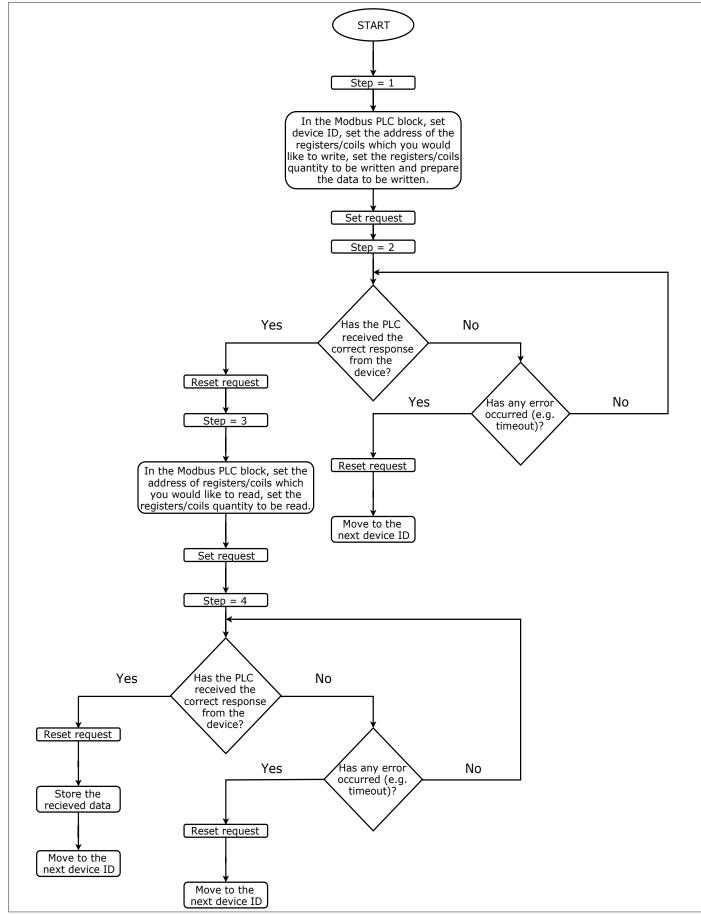
Figure 5 PLC Algorithm
