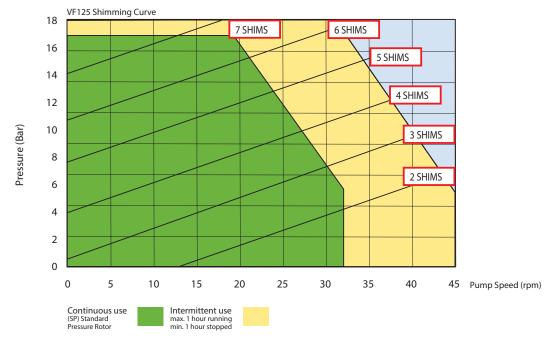
For product temperatures above 149°F and/or viscocity above 2000 mPas use one shim less than shown
