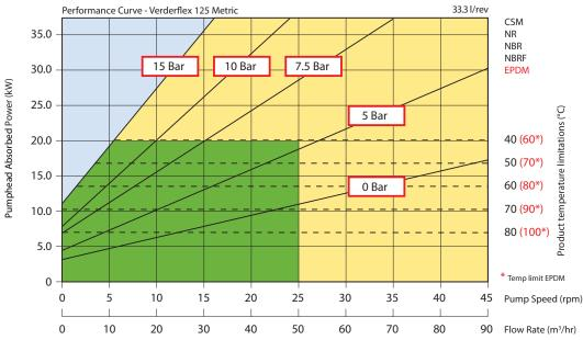
Displacement 33.3 l/revolution, Capacity is speed x 2.0 in m³/hr Minimum starting torque required: 7000 Nm Maximum peak power +27%
